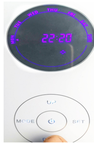
Step 2: press Down button till hour into 22
