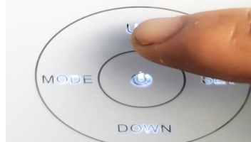
Step 5: press UP button to adjust into 20
