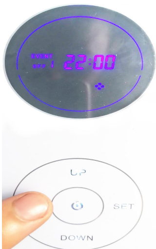
Step 1: press MODE button till " EVENT 1 off", (stop working time )
