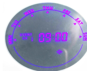
Step 3: press UP button, adjust hour into 9
