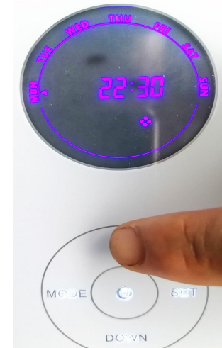
Step 4: press UP button till minutes into 30
